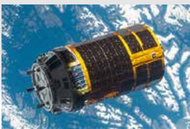
H-II Transfer Vehicle Automated cargo spacecraft used to resupply the International Space Station.
